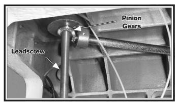
Figure 45. Lower leadscrew and pinion gears.
